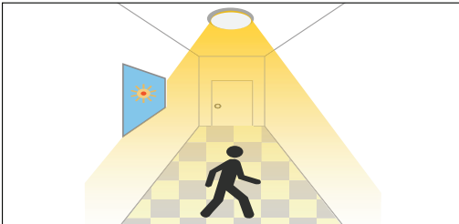
When motion is detected, the sensor will turn the fixture to 100% brightness.
